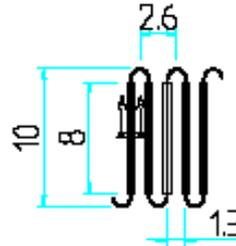
Figure 8: detail of fin spacing
