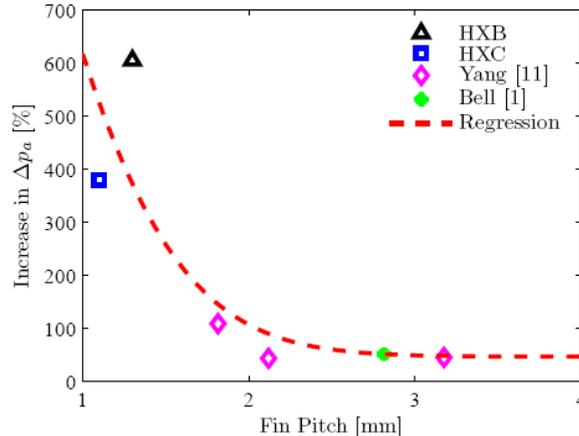
Figure 12 : Increase in air-side pressure loss as a function of the fin space with the injection of  $1612.5 \text{ g/m}^2$  of standard ASHRAE dust [11].
