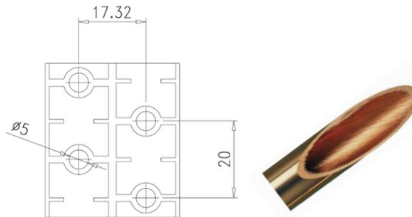
Figure 1 : new coil geometry TURBOFIN 5
