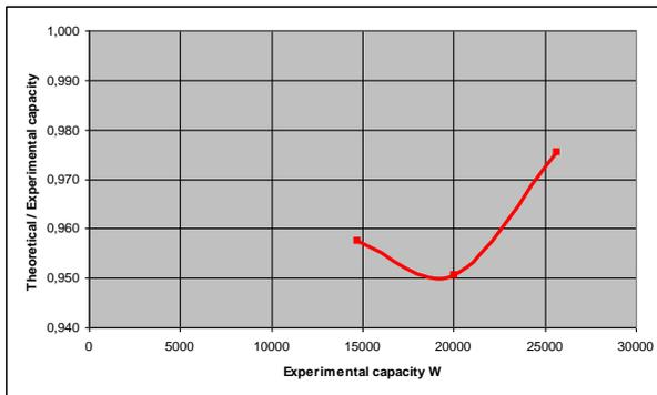
Figure 5 – deviation between calculated and measured capacity (optimized tube)
