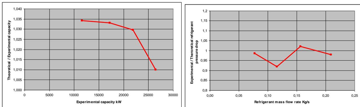
Figure 4a – deviation between calculated and measured capacity (standard tube)
