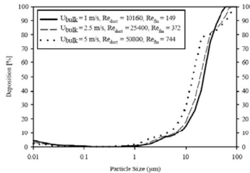
Figure 11 :Modelled deposition as a function of Bulk air velocity on 4,7 fin/cm heat exchanger
