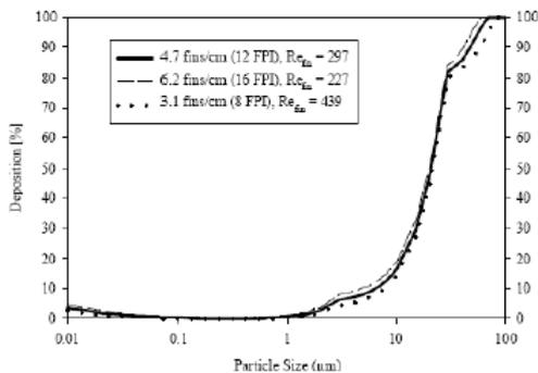
Figure 10 :Modelled deposition as a function of Fin Spacing for a Bulk air velocity of 2m/s
