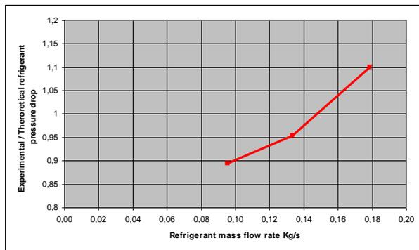
Figure 6 – deviation between calculated and measured refrigerant pressure drop(optimized tube)
