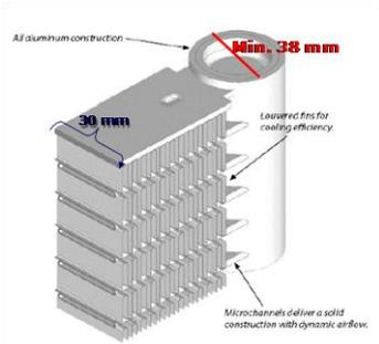
Figure 7 : drawing of Micro channel parallel flow
